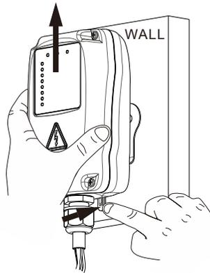
Remove the two components (shown on the right with arrows pointing to them) when the 380~400VAC or 410~460VAC power transformer is used.
