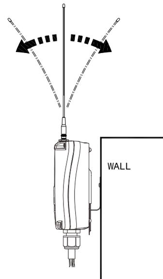
Secure the mounting bracket to the wall or equipment via two screws (not provided with the system). Slide down the receiver along the guided track to secure the receiver to the mounting bracket (see below). Make sure the screws are tightened after installation.
